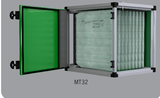
The Camfil GlidePack® MultiTrack housing is a multi-stage air filter housing with adaptable tracks to apply a variety of pre and final filters for superior indoor air quality in virtually any application. The housing may also be reconfigured in the field for upgrades or to adapt the latest air filtration technology.
